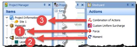
2. Select **Force 1** in the **Project Manager** and, in the **Property Inspector**, change its **Level** (under **Location > Absolute Position**) to 1.75 m – the **Depth** will change to –1.75 m as you do this (the change in level is necessary to place the force on top of the pile cap). Change the force’s **Fx** value to 2000 kN and its **Fz** value to 20 000 kN – the **Resultant** will change to 20 099.75 kN.
