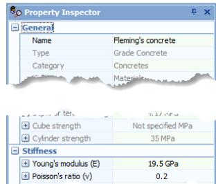
4. In the **Property Inspector**, change the **Length** of the new pile to 12.2 m and its **Shaft diameter** to 775 mm (its **Base diameter** will automatically increase to 775 mm). Finally, select Fleming's concrete in the **Material name** box.
