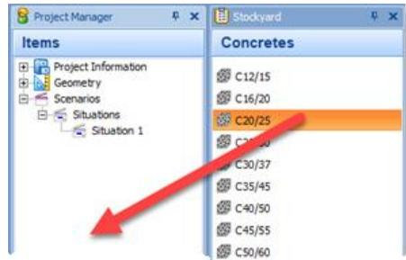
(where it will appear as **Concrete 1**, under the heading **Materials > Concretes**).
