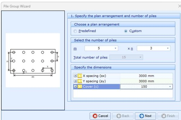
3. Click **Next** to display page 2 of the Wizard. Choose (Cast-in-place Concrete) Bored Pile as the **pile type**.
