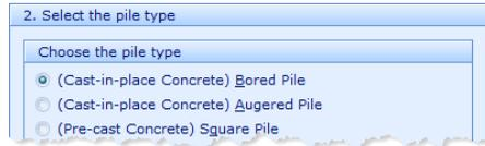
4. Click **Next** to display page 3. Change the **Concrete class** to C20/25 and the **Diameter/Breadth** to 1050 mm. By default, the concrete will be assigned a Young's modulus of 30 GPa.
