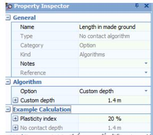
(which is depth of ground that the calculation will ignore when calculating shaft friction).
