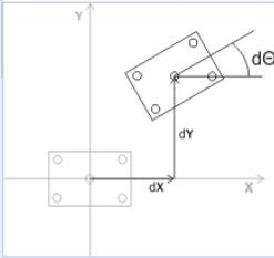
The diagram shows a coordinate system with X and Y axes. A pile group is represented by a rectangle with four circles inside. The centroid is marked with a dot. The distance from the origin to the centroid is labeled 'dX' and 'dY'. The rotation of the pile group is labeled 'dθ'.
