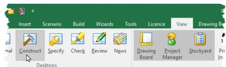
clicking on the **Construct** button. (The **Construction Desktop** displays the **Drawing Board, Project Manager, and Stockyard.**)
