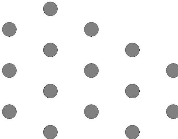
You are interested in the displacements and rotation of the pile cap under a combined vertical load of 50 MN, horizontal loads of 10 MN (in the X direction) and 7 MN (in the Y direction), and moments of 5 MNm (in the XZ
