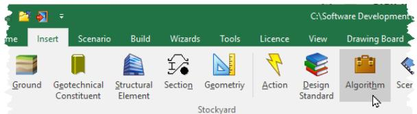
1. Open the **Stockyard's Algorithms** group by selecting the **Insert** tab on Repute's ribbon and then clicking on the **Algorithm** button.
