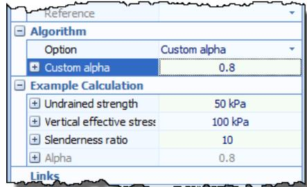
field. Enter a value of 0.8 into the **Custom alpha** box, whereupon **Algorithm > Option** will automatically change to Custom alpha.
